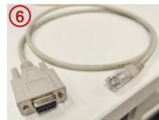
DB9(母头)转RJ45, 串口连接到 X21
